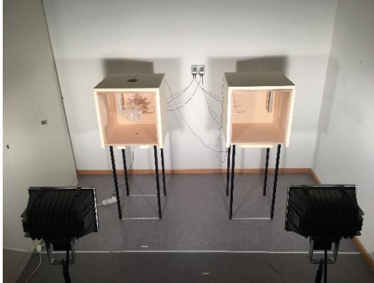
Figure 7: Experimental set-up for thermal cycling
