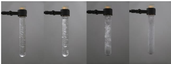
Figure 2: Solidification of bio-based PCM during 10h; crystallization by conduction in contact with containment cooled by the surrounding air
