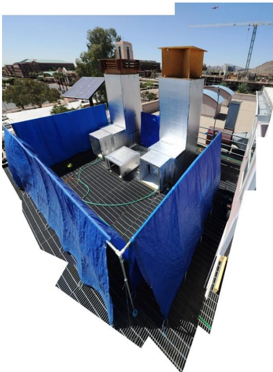
Figure 4: Photo of final experiment setup from southeast corner. Left: hybrid tower, right: single stage tower.
