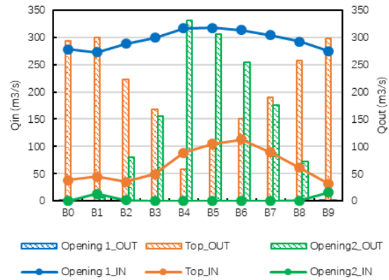
Figure 9: Air flow rate at opening1, opening2 and top boundary for different type B design cases.
