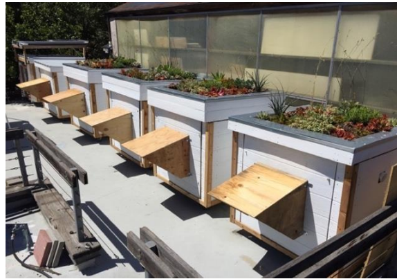
Figure 1: View of the Test Cells with Shade
