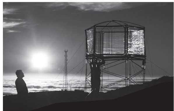
Figure 3. FOGHIVE© test in Atacama Desert, Chile (2014). Source: author, 2018
