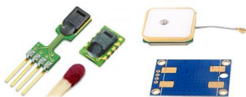
Figure 1: Temperature and Relative Humidity Sensor (SHT75) and GPS Module (Serial NEO-6M, GY-GPS6MV2).
