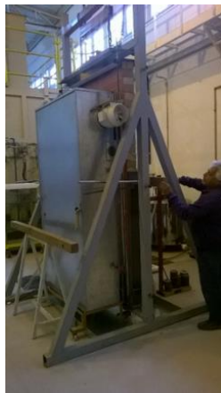
Figure 4: Apparatus for heat and shock test and position of thermocouples.
