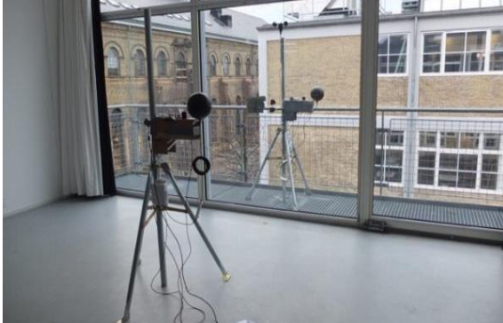
Figure 2: Overview of the stations in the test room (P2 indoor and P3 outdoor) during measurement's phase.
