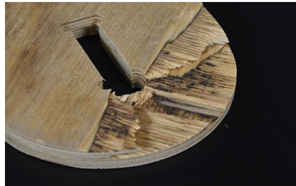
Figure 8: Plywood veneer layers separating on the 'X-Lock' component at a mortise connection.
