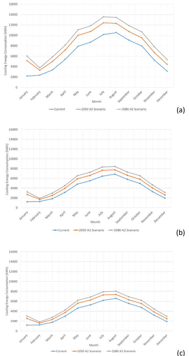
Figure 8: the changes in monthly cooling energy consumption for the base case villa (a), code 1 villa (b) and code 2 villa (c) under the current climate and future climate change (A2 scenario).
