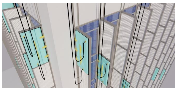
Figure 2: Representation of BICC moveable cleaning chambers
