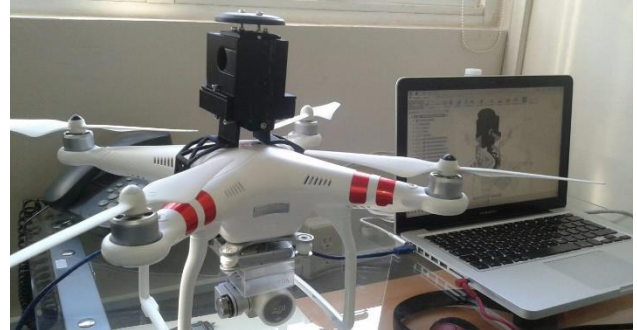
Figure 2: Drone and its superior sensor support system.
