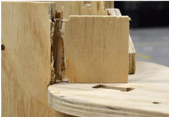
Figure 7: Failure of a perimeter span element of the X-Frame system due to variations in material thickness.
