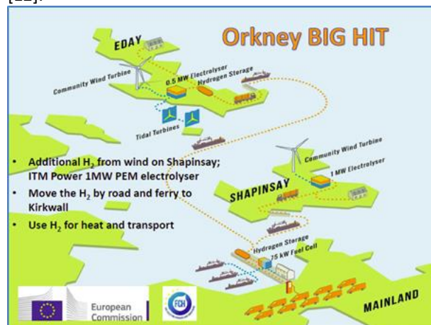
Figure 5: BIG HIT Building Innovative Green Hydrogen Systems in an Isolated Territory: a Pilot for Europe (2016-2020). The schedule shows the combination of wind energy with hydrogen production and storage [12]
