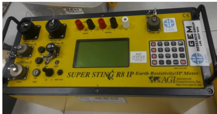
Gambar 3.6 Alat SuperSting R8/IP
