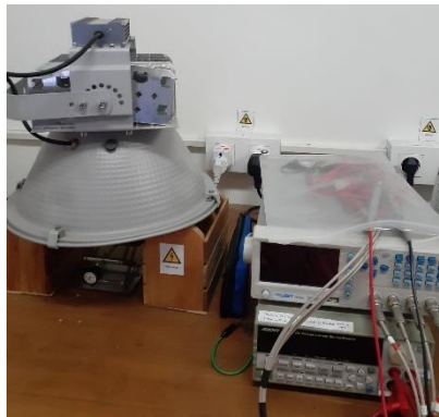
Gamba 3.17 Solar Standard Simulator
