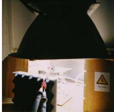
Gambar 3.12 *Standard Solar Simulator 1,5 AM Filter 100 mWcm<sup>-2</sup>*
