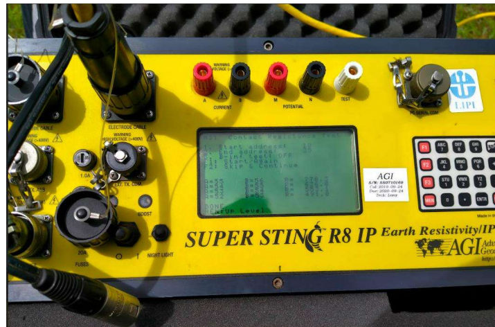
Gambar 3. 5 Alat Pengambilan Data Geolistrik ( Super Sting )
