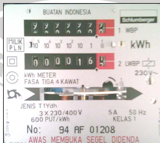
Gambar 3.1 Name Plate kWh Meter 3 Fasa 4 Kawat
