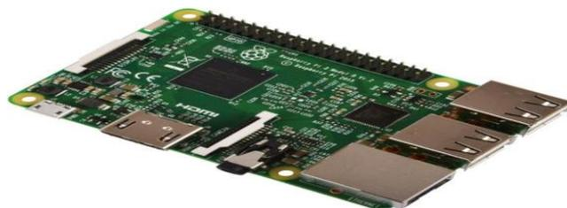
**Gambar 2.1 Raspberry Pi 3 Model B V1.2**
