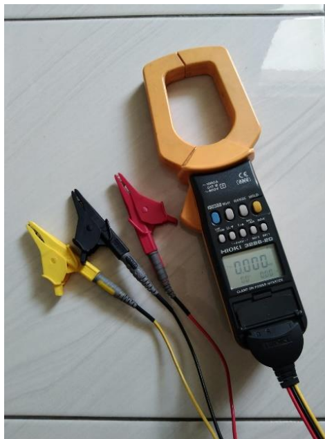
Gambar 3. 3 Clamp on Power Hitester 3286-20
