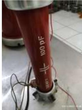
Gambar 3.6 Kopling Kapasitor 100kV-100pF
