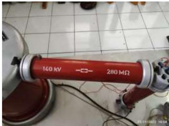
Gambar 3.5 Resistor Pembatas 140kV-280M $\Omega$
