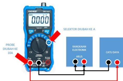
Gambar 3. 18 Prosedur pengukuran arus *input*
