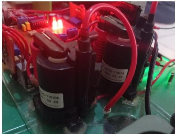
Gambar 3. 11 *Transformator flyback tipe BSC25-T1010A*
