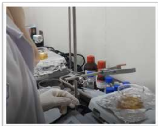
Gambar 3.14 Proses Memanaskan Oil Bath di Magnetic Stirrer
