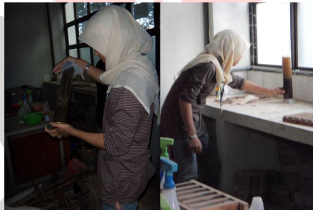
Gambar 3.2. pengujian kadar lumpur agregat halus
