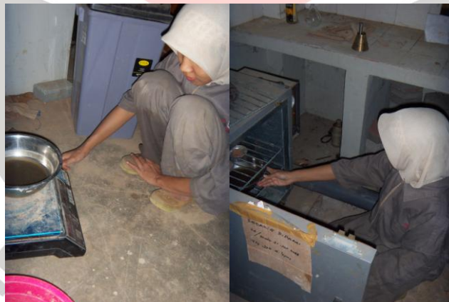
Gambar 3.3. pengujian kadar air agregat
