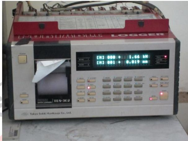
Gambar 3.18 Portable Logger
