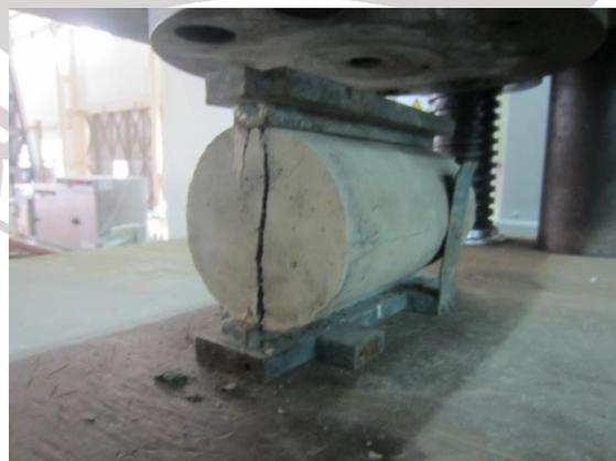
**Gambar 3.14** Pengujian *Splitting* Mortar
