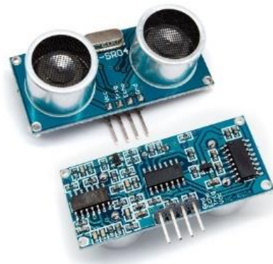
Gambar 3.5 Sensor Ultrasonik HC-SR04 (Sumber : www.shopee.co.id )
