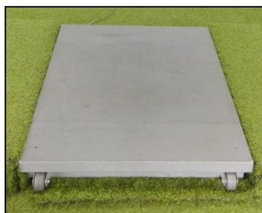
Gambar 3.2. AMTI 3D Force Platform
