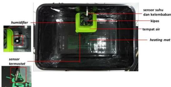
**Gambar 3.4.** Skema Alat Germinator
