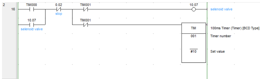
Gambar 3.8 Implementasi selenoid valve
