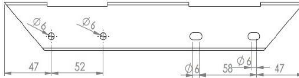
Gambar 3.13 Ukuran drill hollow 1
