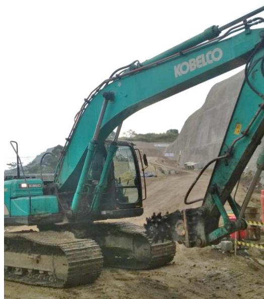
Gambar 3.2 *Excavator Rotary cutter*
