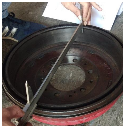
Gambar 3.7 Mengukur Diameter Tromol
