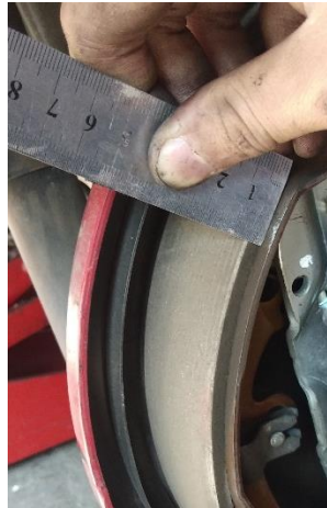
Gambar 3.8 Mengukur Ketebalan Lining Brake Shoe
