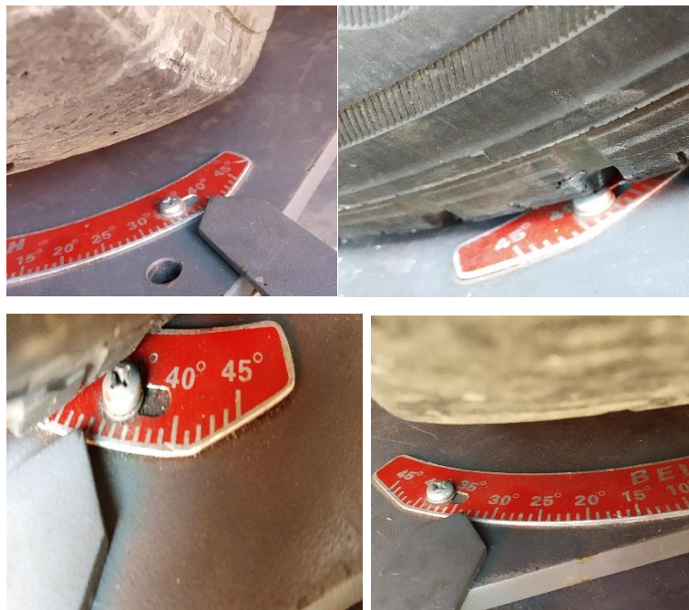
Gambar 3.0.2 Pengukuran Turning Radius
