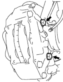
Gambar 3.3 Melepas Disc Brake Cylinder Assembly (Sumber: Repair Manual Toyota Fortuner 2011)
