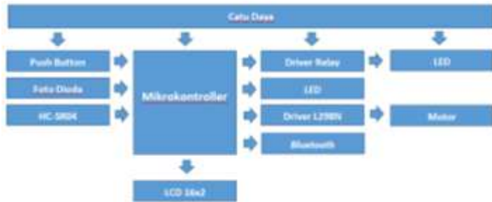
Gambar 0.2 Diagram Block Desain Hardware Training Kit Robotik
