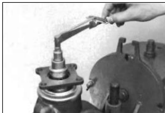
Gambar 3.7 Pemeriksaan Differential Drive Pinion Total Preload (Sumber: Toyota, 1965, hlm. 5-23)
