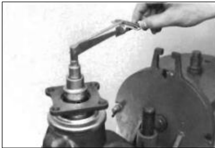
Gambar 3.6 Pemeriksaan Differential Drive Pinion Preload (Sumber: Toyota, 1965, hlm. 5-23)
