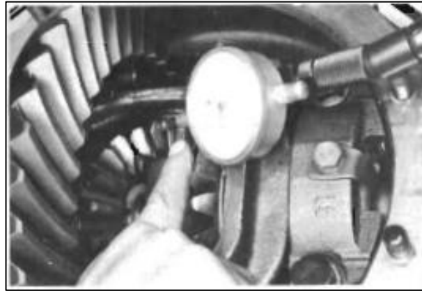
Gambar 3.3 Mengukur Side Gear Backlash
