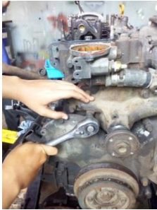
Proses melepas Water pump katup Thermostat
