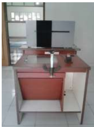
Gambar 3. 2 : Digital-Type Speed Anticipation Reaction Tester (sumber: peneliti)
