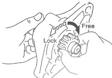
Gambar 3.18 Memeriksa putaran pinion gear (Sumber: Toyota: 1996, hlm. ST-20)
