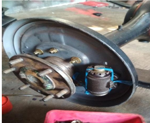
(Gambar Error! No text of specified style in document..10 Keadaan silinder roda terpasang ke backing plate . Tanpa karet boot)
