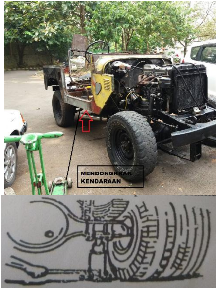
(Gambar Error! No text of specified style in document..1 Medongkrak kendaraan ) (Toyota Astra Motor, New Step 1 1996:5-58)
