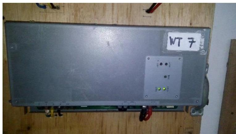
Gambar 3.8 Wind turbin Controller (foto Pribadi)
