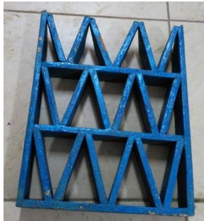
Gambar 3.6 Peredam energi grid triangles tipe 3
