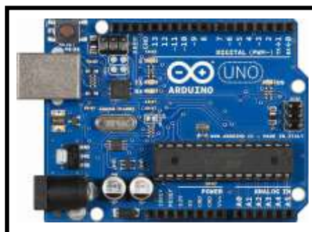
Gambar 3.3 Arduino UNO (Sumber : roboteshop.com)
