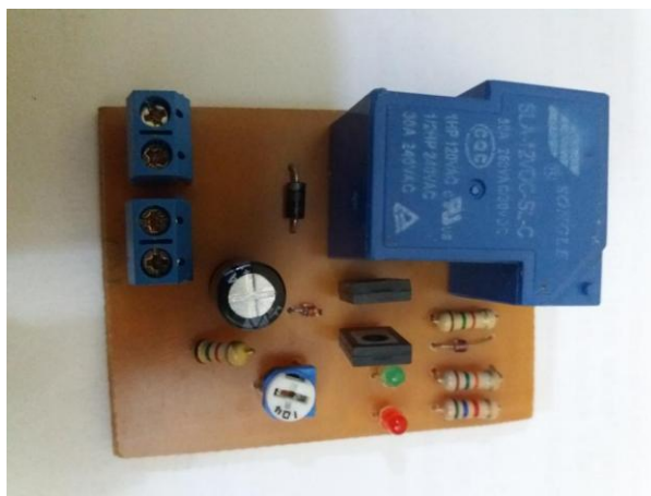
Gambar 3.6 Rangkaian Automatic Battery Charger
