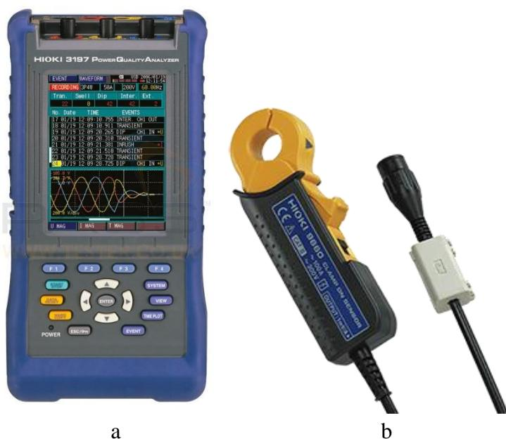
Gambar 3.4 (a) *HIOKI 3197 Power Quality Analyser* dan (b) *Clamp On Sensor 9660*
