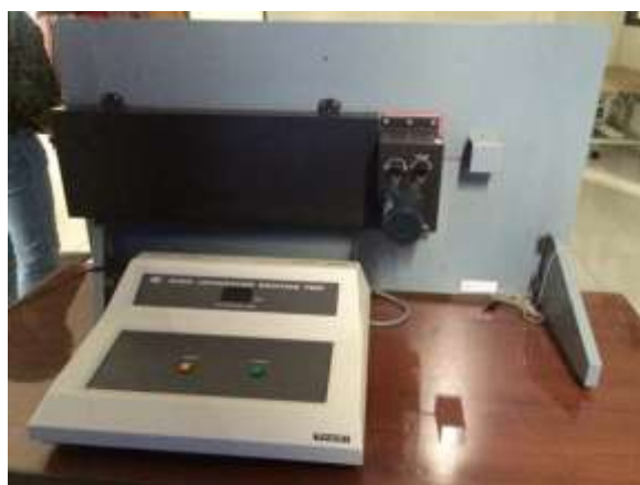
Gambar 3.3 Tampak Belakang Digital Speed Anticipation Reaction Tester
