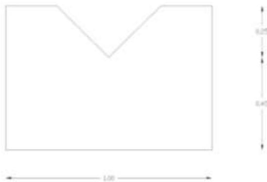
Gambar 3. 5 Geometri V-Notch Weir 3
