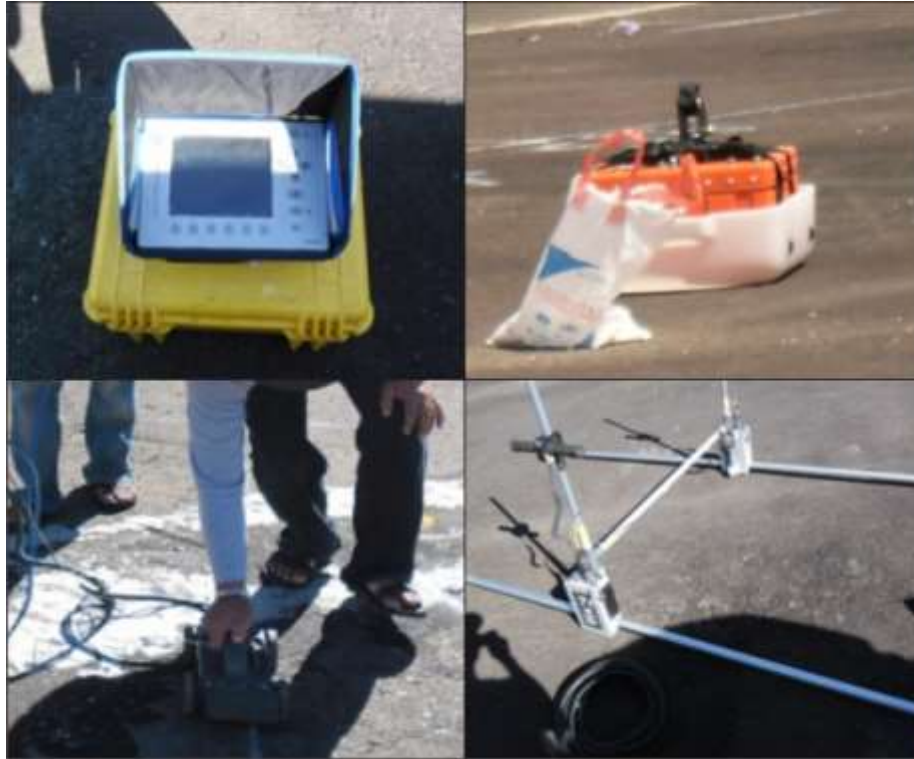
Gambar 3.2. Peralatan GSSI SIR 3000
