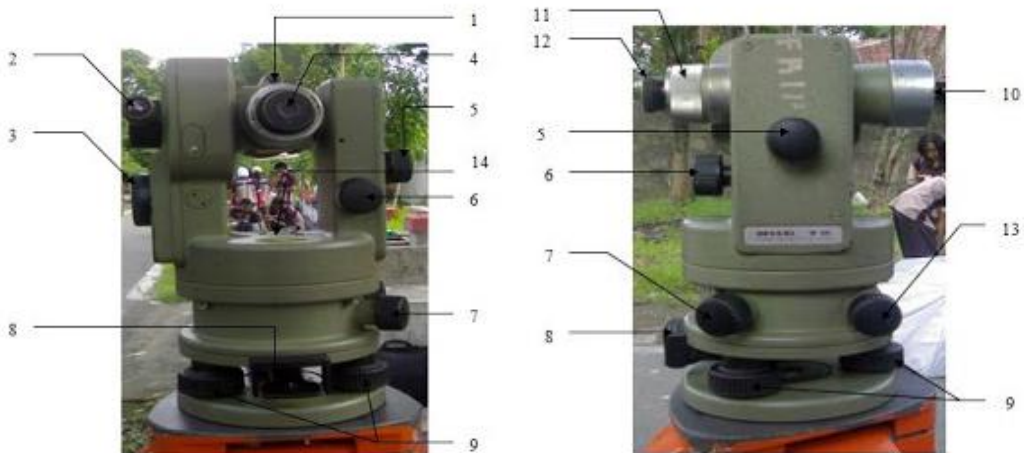
Gambar 3.2. Bagian-bagian Thodolite Wild T0
