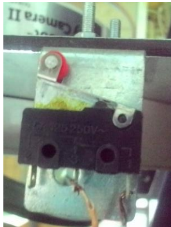
Gambar 4.1 Sensor Limit switch
