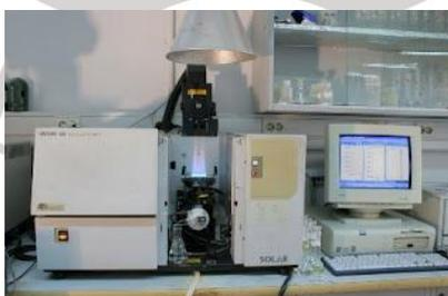
Gambar 3.3 *Atomic Absorption Spectrophotometry* (AAS)
