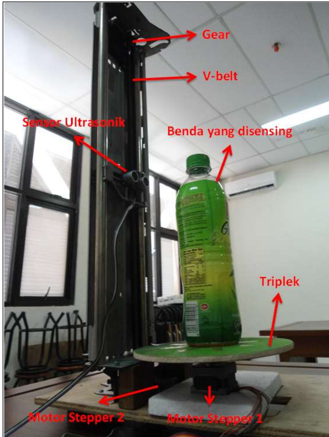
Gambar 3.2 Sistem mekanik scanner 3D.
