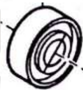
Gambar 3.10 Bearing/Radial Ball (Sumber : Daihatsu, 2007 : D2-17)
