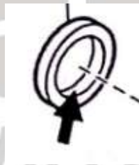
Gambar 3.13 Oil Seal (Sumber : Daihatsu, 2007 : D2-17)
