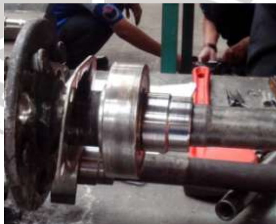
Gambar 3.7 Retainer dan bantalan/ bearing
