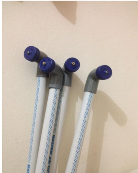
Gambar 4.2 Rangkaian 2 pasang sensor Phototransistor dan 2 pasang laser dioda
