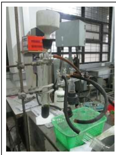
Gambar 3.2. Proses filtrasi dye Cordyline Fruticosa
