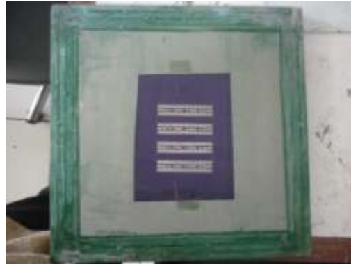
Gambar 3.11 Pola Filter Diatas Screen
