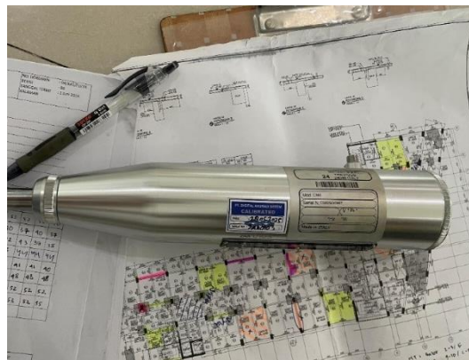
Gambar 3. 3 Alat Rebound Hammer Test
