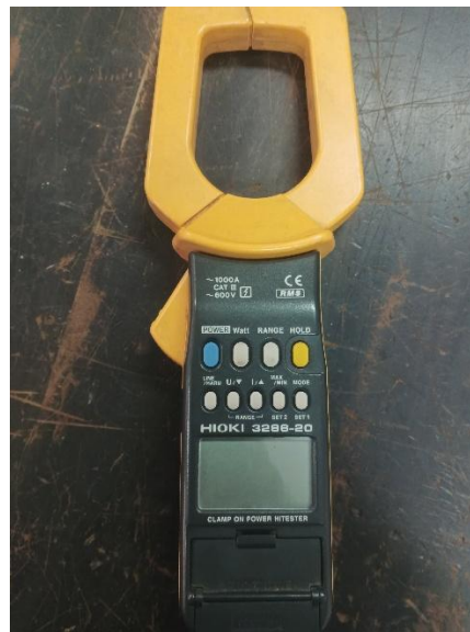
Gambar 3. 7 Clamp On Power Hitester Hioki 3286-20
