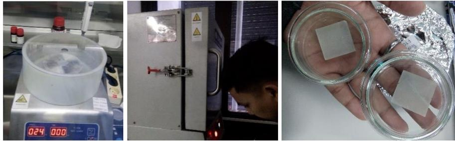
Gambar 3.5 Proses Deposisi  $\text{TiO}_2$
