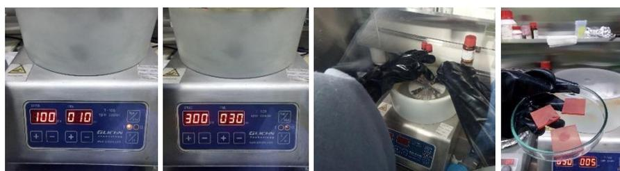
Gambar 3.7 Proses Deposisi Perovskite CsPbIBr<sub>2</sub>
