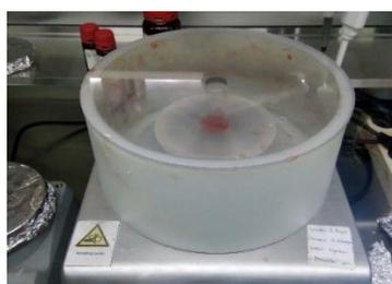
Gambar 3.9 Proses Deposisi Spiro-OMeTAD
