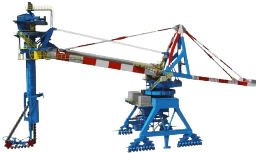
Gambar 5. 1 Alat *Continuous Ship Unloader (CSU)*
