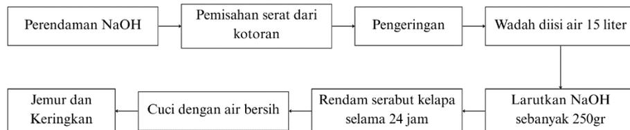
Gambar 3. 2 Flowchart Perendaman NaOH (soda api)
