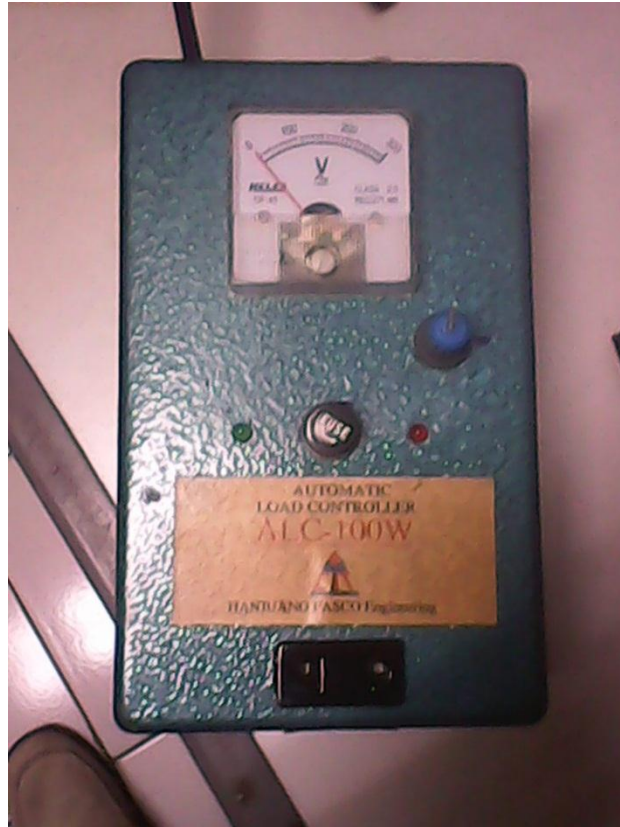
Gambar 3.13 Automatic Load Control
